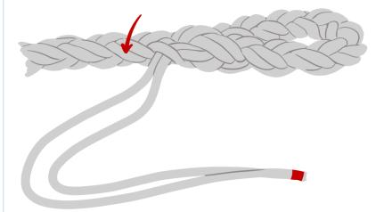
**Step 7:** Pull it snug, and you'll see the pattern to follow henceforth: over one strand; under the next. It's acceptable to go under-two, over-two, but that makes a bulkier splice.
