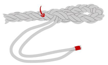
**Step 5:** The strand pair should look like this, emerging from between two strand pairs on the standing part. Other pairs not shown, for clarity.
