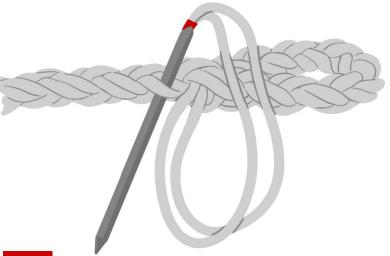
**Step 6:** Take a fid between the strands of the pair on the standing part, OVER the near one, UNDER the offer one. Follow with the two strands.
